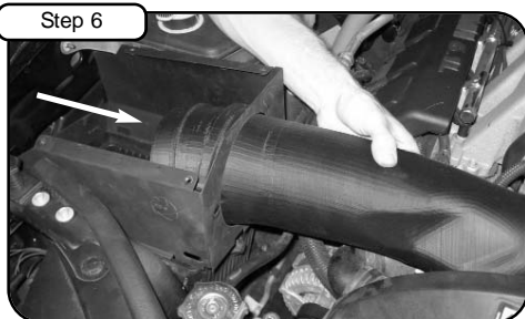
Install housing into position of OE upper airbox and re-clip to bottom of housing. Install tube through housing.
