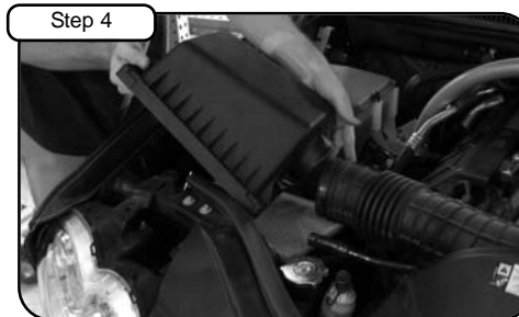
Loosen clamp at air box and un-clip upper half of air box and remove. Also, remove OE intake tube.
