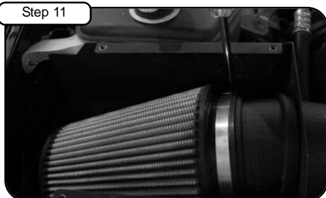
Re-connect air temp sensor harness. Install air filter and tighten using 5/16" nut driver.
