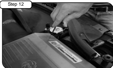
Install cover to housing with button head screws provided and tighten using 5/32" allen key.
