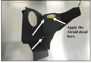
4. Create the panel assembly. Join the Front (#5) and Rear (#6) panels together using the two #6-32 Screws (#18), #6 Flat Washers (#16), and #6 Kep Screws. (#17). Note: The Tab on the Front Panel is to be behind the Rear panel when properly installed.
