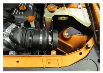
**15.** Install the Intake Tube into the Hump Hose and factory intake tube. When properly installed the location lug in the factory tube will mate with the notch in the Airaid Intake Tube. Tighten the clamps and connect the crank case breather to the Intake Tube.
