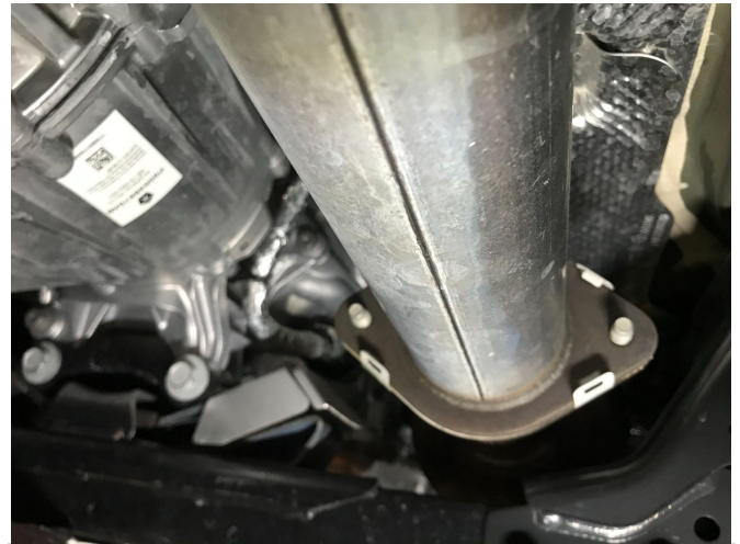
Detail 4: Passenger flanged catback connection
