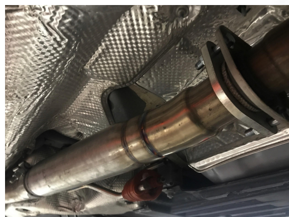
Detail 9: Resonated inlet to X-pipe with hanger installed
