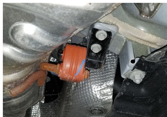
Detail 6: Middle resonator hangers.
