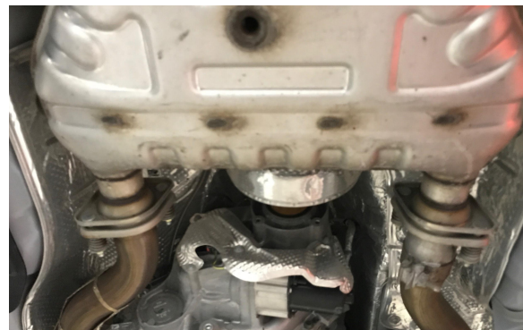
Detail 5: (4) nuts at catback connection
