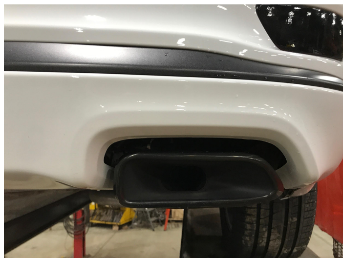
Detail 12: Left muffler assembly with SW round tip installed
