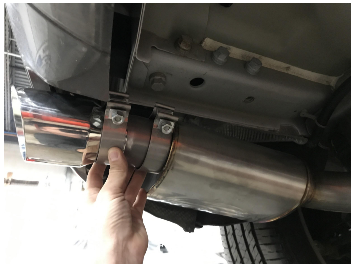
Detail 12: Left muffler assembly with SW round tip installed
