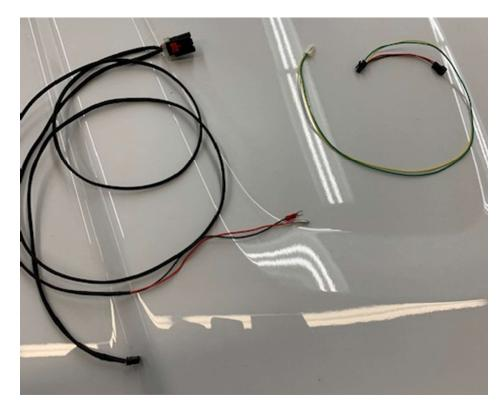
Next, we need to pass the 3-pin connector that separated the interior and exterior harnesses through the firewall. On most vehicles (2011 Charger pictured) there is a body harness grommet on the passenger firewall. This grommet is dual wall with an interior and exterior layer. Cut/puncture through it and pass the harness through. Pictured below we had the red/black/white wires shown as a pulling tool, as we taped the SRV harness to them to pull the connector through the grommet.
