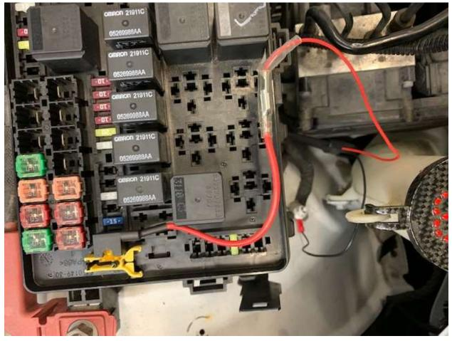
Lastly, Plug the harness into the SRV valve itself. Tie-wrap the harness to secure it away from engine hot or moving parts.
