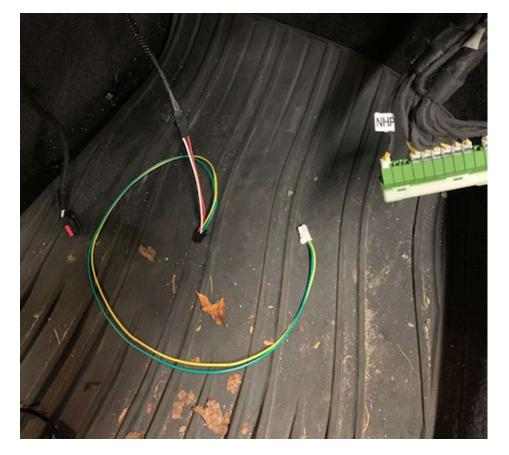
The 6 pin black plug plugs into the SRV controller box (not shown above).
