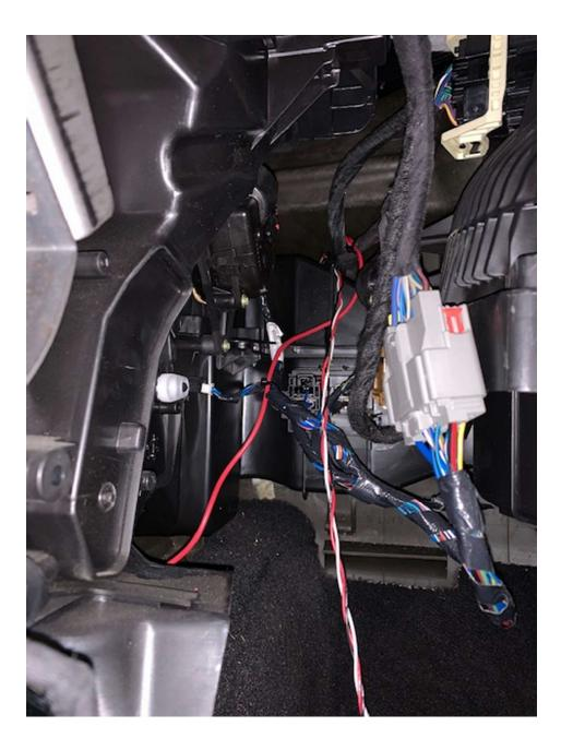
We re-join the interior and exterior harnesses. The 2 pin white connector plugs into the GREEN CAN-C Star connector, found on Powernet vehicles only. On most cars it's located behind the glove box; most trucks it's located by the steering column. Plug into any available slot.
