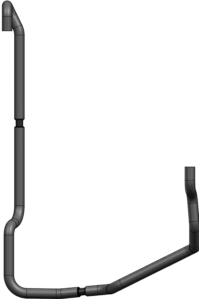
56-0006 Heat Exchanger to Manifold
